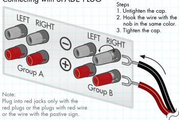
\*Note: The back panel may be placed different on actual machines; Please turn off the power and unplug the equipment before changingthe wiring configuration; Miss-connecting may damage equipments.
